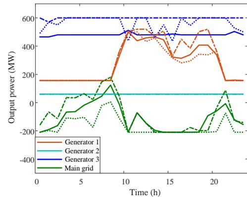
Fig. 4. The reference (solid lines), worst-case (dash-dotted lines), and actual (dashed lines) power outputs of controllable generators and power purchased from the main grid.
