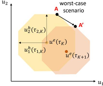
Fig. 2. Illustration of (23). The yellow and orange regions are the uncertainty sets in the  $K$  and  $K+1$  iterations, respectively. Point A is the worst-case scenario in the  $K$  iteration. When  $u^e$  and  $u^h$  changes with  $\tau$ , (23) moves point A to point A', which is a vertex of the new uncertainty set.
