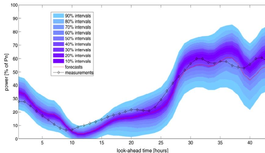
**Figure 2:** Example of 2 day-ahead forecasts of wind power for a region in the Northern part of Denmark. These forecasts give both the expected power production and the probability distribution of power production for each look-ahead time.
