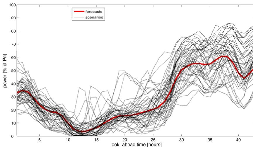
**Figure 3:** Example of a set of 2 day-ahead statistical scenarios of wind power production corresponding to the probabilistic forecasts of Figure 2.
