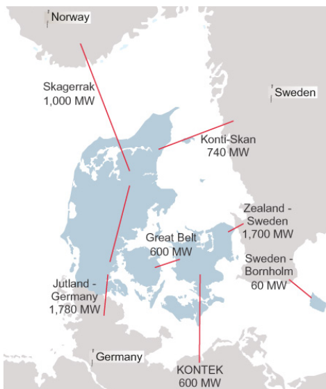
Fig. 1. Interconnection to the Danish power system as of 2014. In 2015, the Skagerrak transmission facility connecting Denmark and Norway was upgraded to 1.7GW. (source: Energinet.dk).
