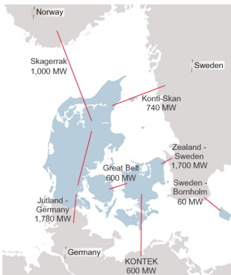
Fig. 1. Interconnection to the Danish power system as of 2014. In 2015, the Skagerrak transmission facility connecting Denmark and Norway was upgraded to 1.7GW. (source: Energinet.dk).
